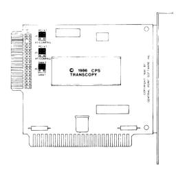
You need to configure it now for your IBM PC/AT computer. To do this, carefully remove each of the plastic jumpers one at a time and connect them to the middle and end pins closest to the AT/Compaq lettering on the board. When you're done, it will look like this:
