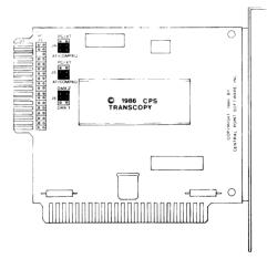
Next, you need to reinstall the cable on the Option Board. Take the cable you just removed from the board and plug it into the end of the board (the gold-plated connector labeled J3). The red line on the cable should be closest to the top of the Option Board. Note that this is different from the way the cable was installed on the board originally. This is necessary as the cable coming from your disk
