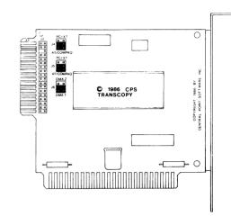
The drive cables will connect to the J2 connector with the red line closest to the bottom of the Option Board. Connect the remaining cable to the J3 connector with the red line down. The other end of this cable connects to the Tandy motherboard. The red line on this cable goes closest to the edge of the Tandy motherboard.
