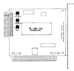
This means the Option Board is currently configured to be installed into an IBM PC or PC/XT. You need to configure it now for your Compaq computer. To do this, carefully remove each of the plastic jumpers one at a time and connect them to the middle and end pins closest to the AT/Compaq lettering on the board. When you're done, it should look like this:
