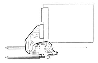
After you have installed the Option Board into slot #2, you have just one connection left to make. The cable that leaves the end of the Option Board needs to plug into the disk controller board at J1 (which is where the floppy disk drive cable used to connect). The red line on the cable should be up, towards the top of the connector on the disk controller board.
